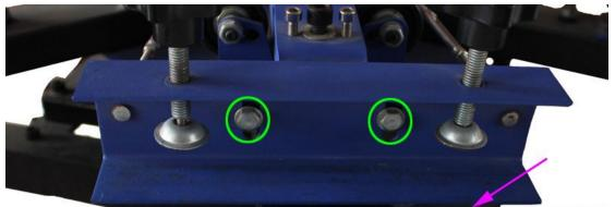
1. Adjusting the two screws to confirm that the bottom line of the printing head will be in paralleled with the printing pallet.
