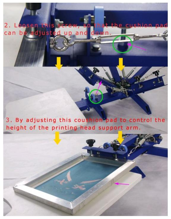
Forth Put down the printing head again to confirm whether it can be easily to be lifted or down easily after installing a screen frame.
