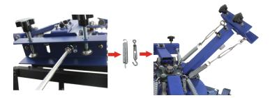
Close Attention: All four arms of printing head have been position-adjusted and all the screws have been tightened before delivery; please do not adjust these screws of the printing head support arms during installation and operation.
