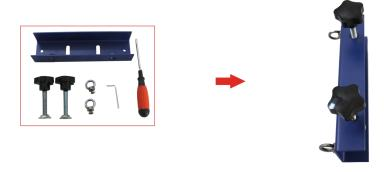
c. Connect the printing head collets and the position collet fastenings by tightening 8 screws.
