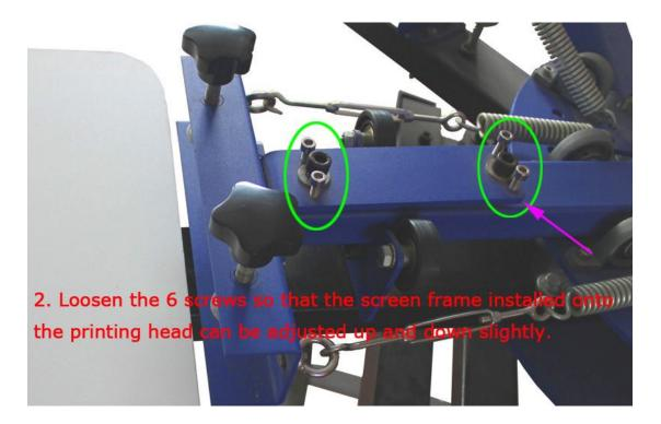
Three Once the 6 screws have been loosened, then swing the screen frame slightly.
