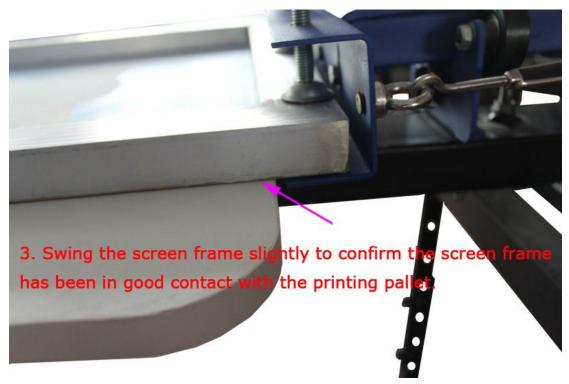
Four While the screen frame has been in paralleled with the pallet, first fix the four small screws slightly; Then fasten the
