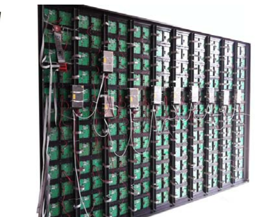
Controller Card LED Module Power Fixed Keel Data Cable 5V DC Wire
