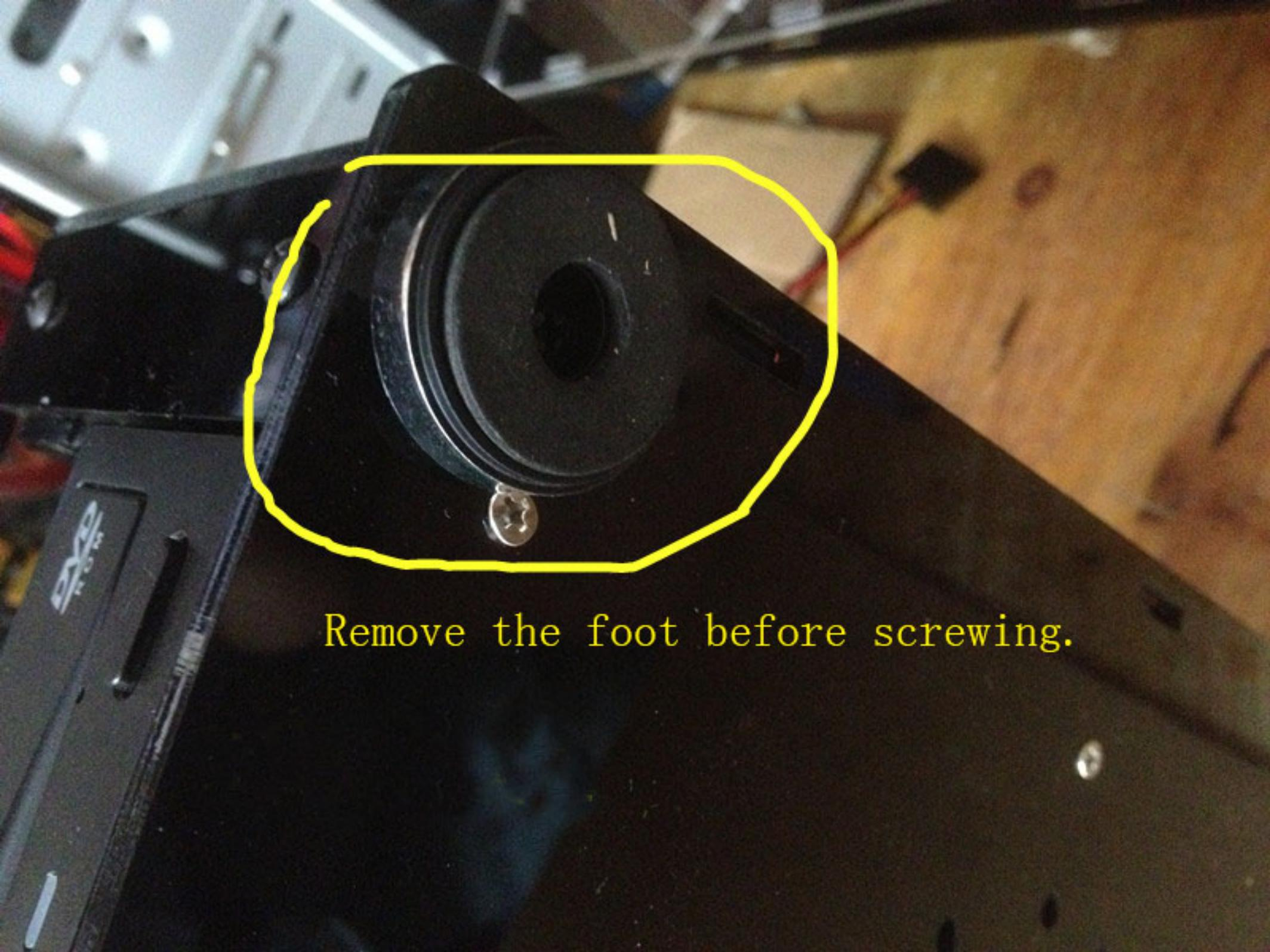
Remove the foot before screwing.
