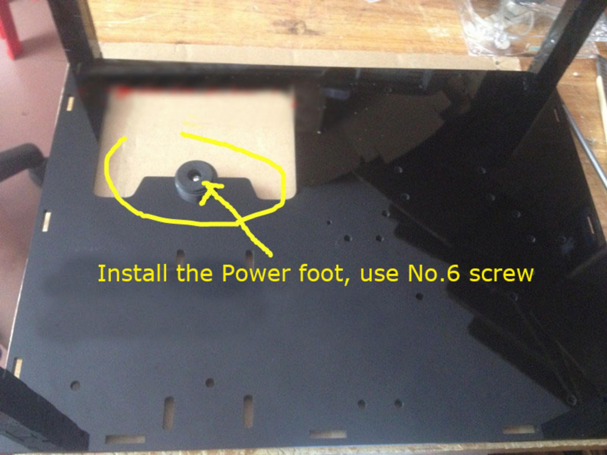
A black metal chassis is shown from a top-down perspective. A power foot, which is a small black cylindrical component with a central hole, is being installed into a pre-drilled hole on the chassis. A yellow hand-drawn circle and arrow highlight the power foot and its location. The chassis has several other holes and slots. In the background, a wooden workbench and a clear plastic bag containing small parts are visible.
