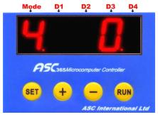
**4) Heating way set:** ((Hint: when the "MODE" is set "4", only set "D3" as "0", other are not the setting functions of this machine and they can't be supported.))
